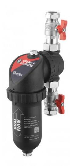
High-performance magnetic filter designed for central heating installations which removes all contaminants (magnetic and non-magnetic) from the installation and effectively stops them inside the device. Dual-flow technology - maximises the efficiency of contaminant capture, and 360 control allows quick and easy installation at any angle on the installation. Set of connection valves are included.
