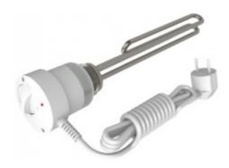
EJK Mini heaters are designed for SG Plus 100, SG Plus 120, SG Plus 140, and ZWU-200/N Plus enamel domestic hot water cylinders and serve as an additional heating element. The heater has a non-automatic temperature limiter, referred to as STB, which protects it from overheating and cuts off the power supply to the heating unit if the temperature controller is damaged.
