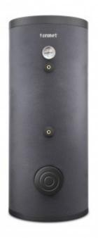
TERMET AQUA 300 I tanks (with a double coiled coil) are intended only for heating, storing and supplying hot water. The device is made of high-quality steel, additionally internal anti-corrosion protection made by the enamelling process. An additional protective element is the protective anode, which is a consumable element and subject to cyclical mandatory replacement (see warranty conditions).
