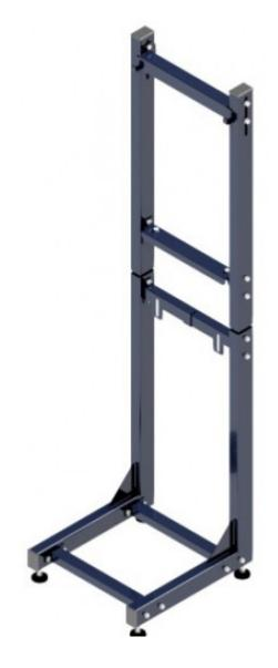
The stand has been designed to facilitate the installation of the Crystal wall-mounted boilers. The construction of the stand enables its quick assembly (using the attached sets of mounting screws) at the final installation site. The system of holes allows for precise adjustment of the boiler height. The stands can be connected in series while maintaining the appropriate chimney spacing (using an additional set of screws and sheets). The frame is available in graphite color.
