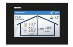
TERMET ST-2801 with Open-Therm protocol ensures intelligent maintenance of the set room temperature by automatic proportional regulation of the prset boiler temperature. Controller enables user to adjust the control algorithm parameters. Big advantage of ST-2801 controller is its colour, large and easy-to-read touch display. It allows for very comfortable operation of the device and modulation of its parameters. Easy flush-mounting in an electrical box (ø60mm).
