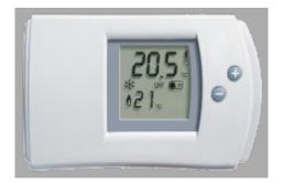
TERMET 1210 is an easy-to-use temperature controller which allows for simple room temperature control. Liquid crystal and clear display indicates on set temperature and informs of a necessity to exchange the batteries. The regulator has his own battery power supply and an operation indicator of heating device.
