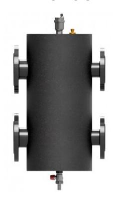
Hydraulic separator is made of steel. It has been designed to separate the boiler pump from the pumps in the system. Hydraulic separator is designed for installation with MK collectors for the total power of boilers in a cascade up to 470 kW (depending on the model).
