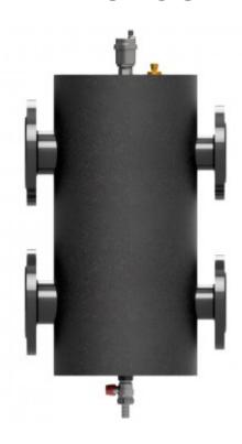
Hydraulic separator (hydraulic coupling) is made of steel. It has been designed to separate the boiler pump from the pumps in the system. Hydraulic separator is designed for installation with MK collectors for the total power of boilers in a cascade up to 470 kW (depending on the model).
