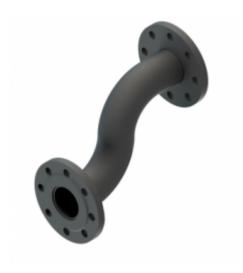
**The S connector** is made of steel. It was designed to reduce the installation height of the cascade distributor. The **set includes one connector** and a set of 4 mounting screws with a gasket. **Two pieces of connector** are required to connect the collector with the hydraulic clutch.
