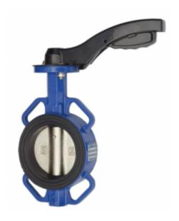
**WX butterfly** valves are designed for shutting off and regulating the flow of cold and hot water. They are used in heating systems, sewage systems and tap water systems (with a stainless steel disc). Short construction, low pressure losses and simple assembly allow for use wherever it is impossible to install a ball valve.
