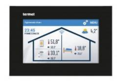
TERMET ST-2801 with Open-Therm protocol ensures intelligent maintenance of the set room temperature by automatic proportional regulation of the prset boiler temperature. Controller enables user to adjust the control algorithm parameters. Big advantage of ST-2801 controller is its colour, large and easy-to-read touch display. It allows for very comfortable operation of the device and modulation of its parameters. Easy flush-mounting in an electrical box (ø60mm).
