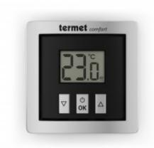
The Comfort Regulator is a wireless temperature controller equipped with a temperature sensor, display and buttons for room temperature control. It provides the Comfort Module with information about the temperature in the zone in which it is located. The controller allows for independent control of up to four radiator heads.
