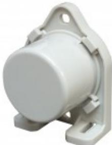
Outside temperature sensor is intended to be mounted outside and gives opportunity to automatically adjust the water temperature in central heating circuit. This adjustment takes place depending on the increase or decrease of the outside temperature. The sensor controls the weather function based on heating curve.
