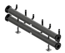
Collector MK 80 - DN 80 is made of steel. It was designed to connect boilers into cascade systems. The factory includes insulation, 2 blind flanges with a socket, 2 bimetallic thermometers, two 1/2" blanking plugs, mounting feet, a set of 16 mounting screws and 4 EPDM DN 80 gaskets.
