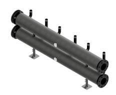
Collector MK 100 - DN 100 is made of steel. It was designed to connect boilers into cascade systems. The factory includes insulation, 2 blind flanges with a socket, 2 bimetallic thermometers, two 1/2" blanking plugs, mounting feet, a set of 16 mounting screws and 4 EPDM gaskets DN 100.
