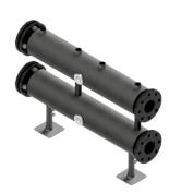
Collector MK 65 - DN 65 is made of steel. It was designed to connect boilers into cascade systems. The factory includes insulation, 2 blind flanges with a socket, 2 bimetallic thermometers, two 1/2" blanking plugs, mounting feet, a set of 16 mounting screws and 4 EPDM DN 65 gaskets.
