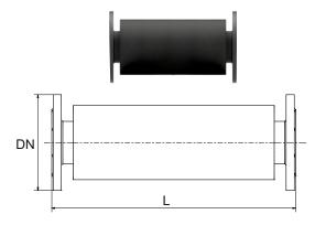
Straight distance connector helps install the basket strainer in pump group systems.
