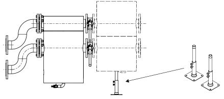
In case of assembly basket strainer with hydraulic separator in the presented configuration brackets included in set with basket strainer should be used.
